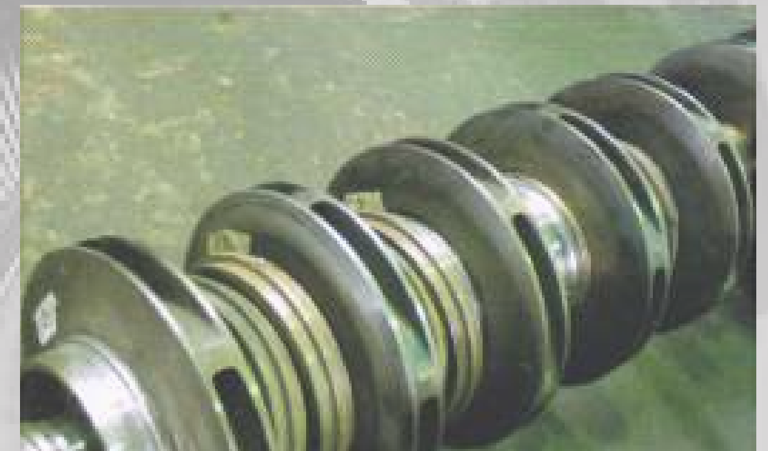
STAGE PUMP ROTOR
